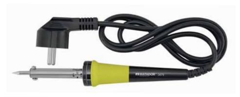
Million times proven universal soldering iron with 40 W for increased heat requirements. Versatile for soldering tasks in the areas of craft / service and hobby. Equipped with a professional permanent soldering tip. ROHS compliant with an operating voltage of 230 volts and a heat-up time of 120 seconds. Maximum soldering tip temperature of 420 °C. Soldering tip diameter 3.10 mm.
