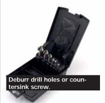
Assortment with 6 powerful countersinks from 6.3-20.5mm, with 90° countersinking angle in a stable plastic case. For countersinking and deburring with three cutting edges for optimal results. According to DIN 335, form C.
