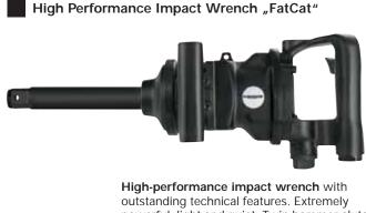
High-performance impact wrench with outstanding technical features. Extremely powerful, light and quiet. Twin hammer clutch mechanism with 6-blades rotor. Cold-insulated, non-slip handle. Ultra light composite housing. Enormous 3.389 N·m loosening torque. Only 96 dB (A) sound pressure level. Only 6.5 kg weight due to composite housing. With long anvil 180 mm (3"). Complete with side handle with mounting kit. Including coupler.
