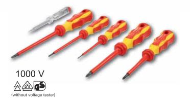
6-pc. set of the most important VDE screwdrivers. With dual compound handles: Yellow, soft and anti-slip grip zone made of TPE plastic for secure hold with maximum pressure. Red, hard turning zone for quick working with low friction. High security through unique identification. Insulated according to IEC 60900:2004.
