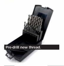
Assortment with 19 high-performance twist drills from 1-10mm x 0.5mm increasing in a sturdy plastic case. Can be used in steel, cast steel alloyed and unalloyed up to 900 N/mm<sup>2</sup> strength, aluminum etc. From Ø 3.0 mm split point according to DIN 1412 C, right-hand cutting with a helix angle of 20 - 30° and the diameter tolerance h8 according to DIN 338.
