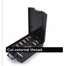
9 pcs. Die set in pre-slit (closed) design from M3 - M12 for cutting external threads in a stable plastic case. For general use, e.g. suitable for steel up to 900N/ mm2. With a diameter tolerance of 2A, 6g for metric ISO threads according to DIN 13.
