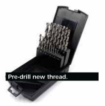
Assortment with 19 high-performance twist drills from 1-10mm x 0.5mm increasing in a sturdy plastic case. Can be used in steel, cast steel alloyed and unalloyed up to 900 N/mm<sup>2</sup> strength, aluminum etc. From Ø 3.0 mm split point according to DIN 1412 C, right-hand cutting with a helix angle of 20 - 30° and the diameter tolerance h8 according to DIN 338.
