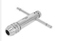
with ratchet and 2-jaw chuck. For all tools with square or hexagon shank (size 1). With Thandle for comfortable work and hardened, exchangeable parallel jaws. For taps and screw extractors M3 - M10 with a clamping range of 4.6 - 8.0 mm.
