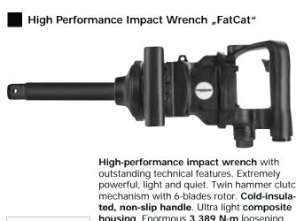
powerful, light and quiet. Twin hammer clutch mechanism with 6-blades rotor. Cold-insulahousing. Enormous 3.389 N⋅m loosening torque. Only 96 dB (A) sound pressure level. Only 6.5 kg weight due to composite housing. With long anvil 180 mm (3"). Complete with side handle with mounting kit. Including coupler.
