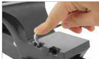
Adjustable spindle guides for backlash-free operation.
